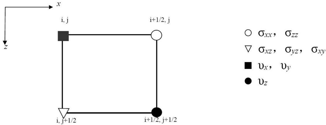
**Figure 1** Grid layout for staggered grid formulation. The indices  $(i, j)$  represent values of the spatial coordinates  $(x, z)$ , respectively.
