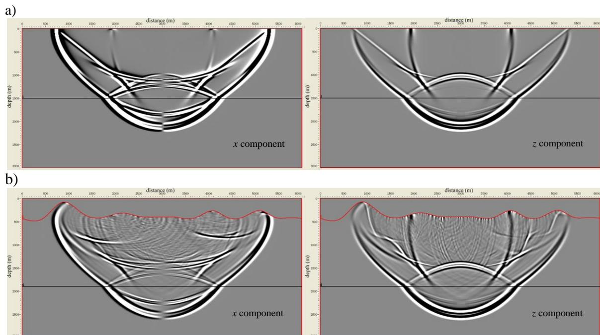
**Figure 3** Snapshots of  $x$  and  $z$  components of particle velocity for elastic anisotropic wave propagation in a complex model. (a) the first simulation. (b) the second simulation.
