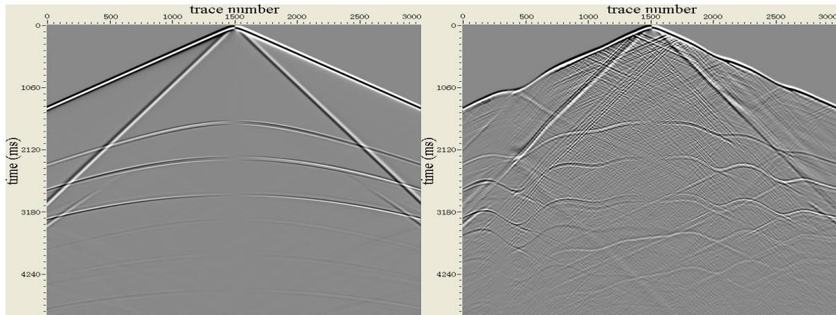
**Figure 4** Seismogram record of the velocity  $x$  components along the free surface in (a) the first simulation and (b) the second simulation.
