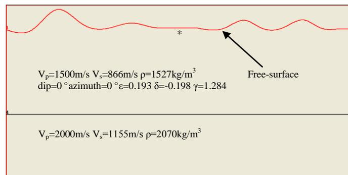
**Figure 2** The irregular free surface model. The star denotes the location of the 30Hz Gauss wavelet source.
