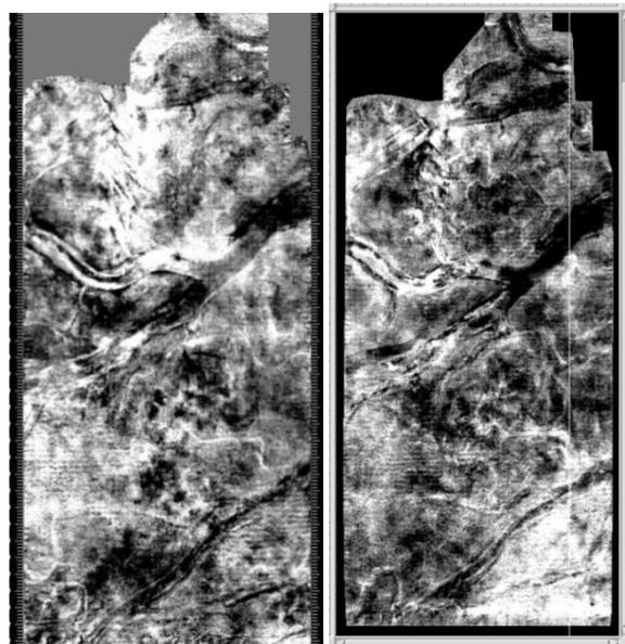
**Figure 4** Seismic time slice (Left: horizon slice; Right: strata slice)
