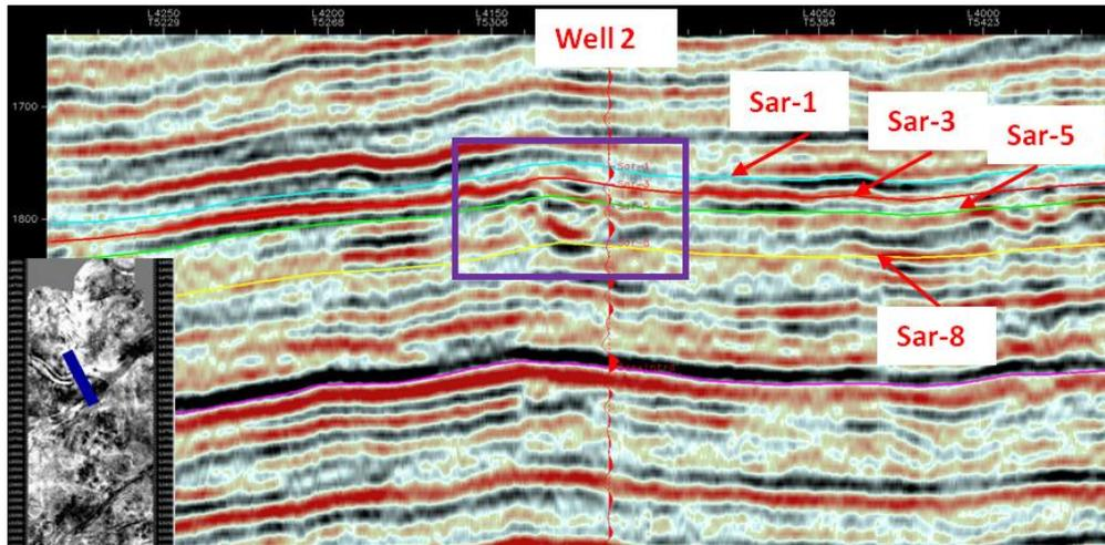
**Figure 5** Seismic profile (in the purple polygon showing the tidal channel through Well 2)
