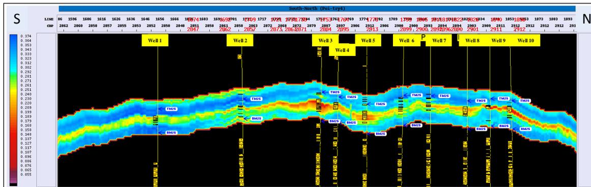
**Figure 7** Inversion result (Poisson's ratio) of M2 result
