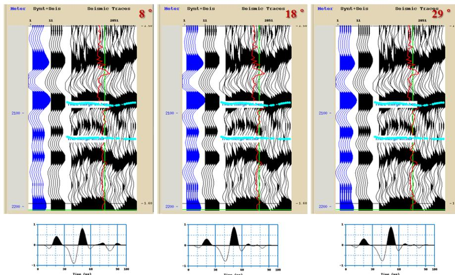
**Figure 6** M2S layer wavelet extraction results for incidence  $8^\circ$ ,  $18^\circ$ ,  $29^\circ$
